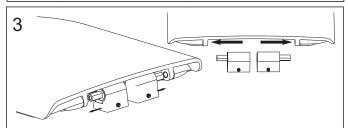
Insert Left & Right Hinge Block fully into holes in seat. Ensure the grub screw fixing hole is at the back.
