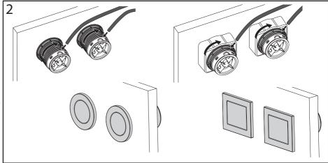
Insert the Button Assembly and ensure buttons are orientated correctly prior to tightening mounting nut from behind. **NOTE**: Rectangular Installations where the thickness of the mounting plate is less than 26mm will require the additional Spacer.
