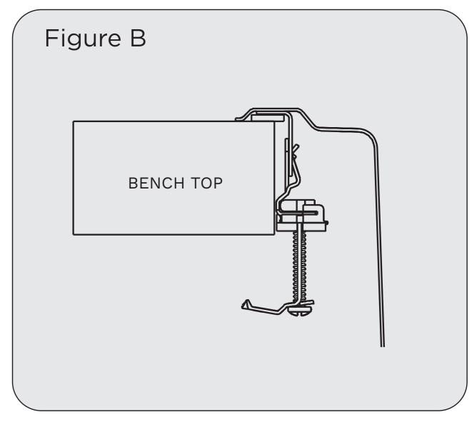
**NOTE: For thin benchtops special** clips (A0167) are available. CUTOUT TEMPLATE DIMENSIONS - 1176 x 476mm To use this cutout template for benchtops, print 1:1 on a large format printer Corner radius 118mm
