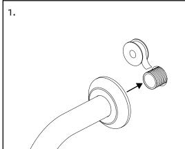
Apply plumbing tape to pipe. Screw arm onto pipe ensuring that the arm ends in the correct position.
