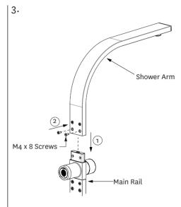
Assemble the shower arm by sliding it onto the top end of the main rail. Secure the shower arm in place with the screws provided.
