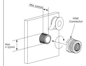
Install a ½" male threaded connection at the recommended height on wall, ensuring that a minimum of 10mm of thread protrudes past the finished wall.
