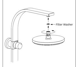
Remove the protective cap from the shower head ball joint and screw the shower head onto the shower arm, ensuring that the filter washer is in place.
