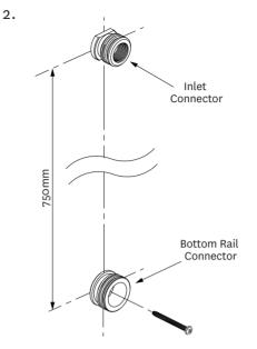
Screw the bottom rail connector to a wall stud vertically in line with the inlet connector and at the correct distance.
