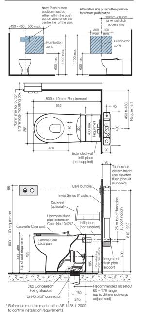
Note: The projection requirements detail on this illustration are for wheel chair access only. The projection requirements for people with ambulant disabilities is 610 to 660mm.
