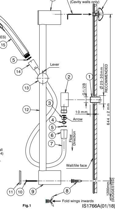
Use a small allen key or nail to spread wings of anchor behind wall
