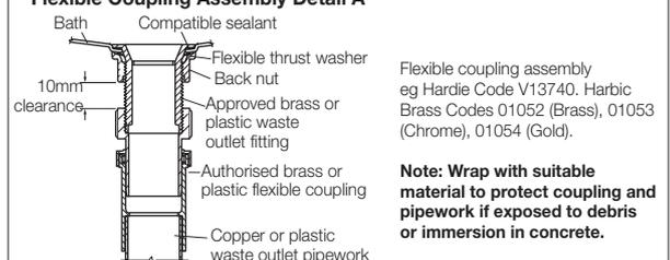
Flexible coupling assembly eg Hardie Code V13740. Harbic Brass Codes 01052 (Brass), 01053 (Chrome), 01054 (Gold).
